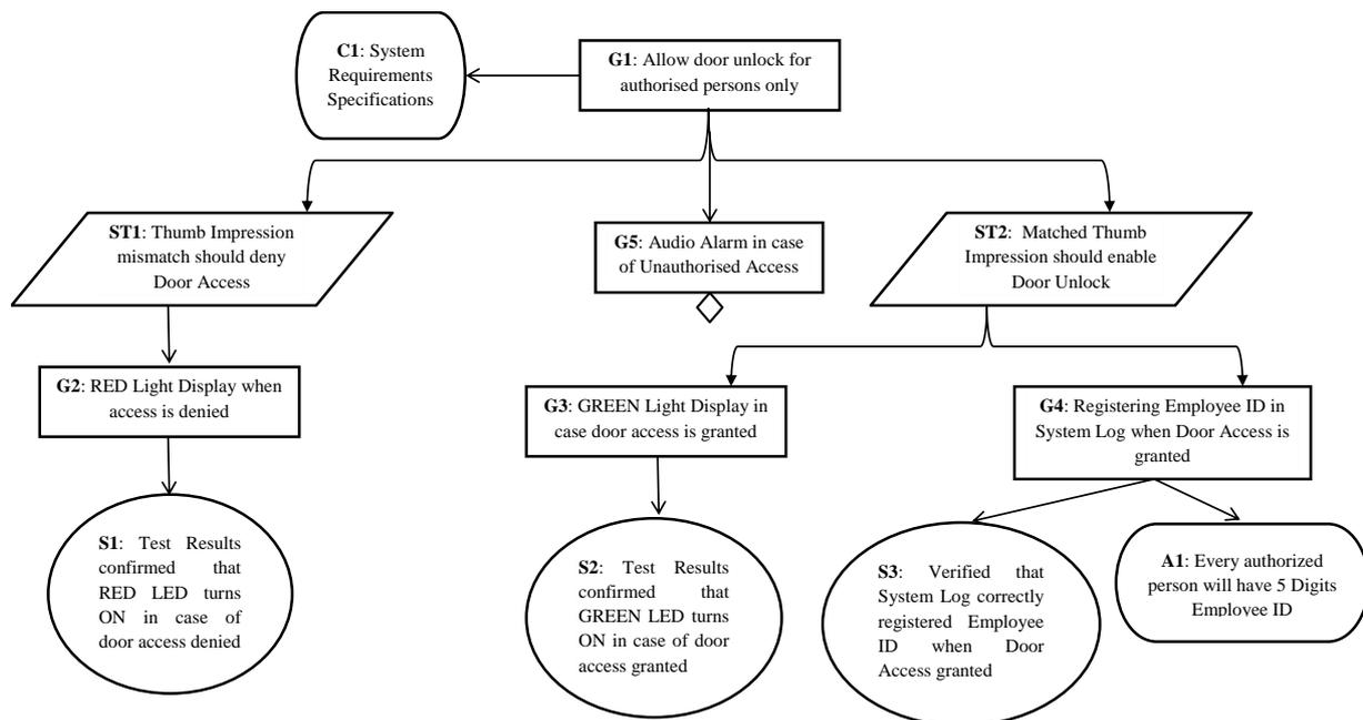
Fig. 2 Assurance Case for Door Access Control Software
